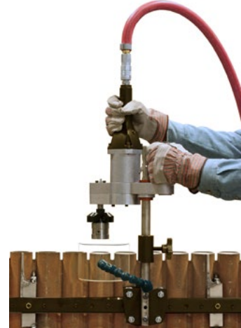
The Track Chassis and Post Assembly's adjustable depth stop ensures all tubes are beveled to the same height.
