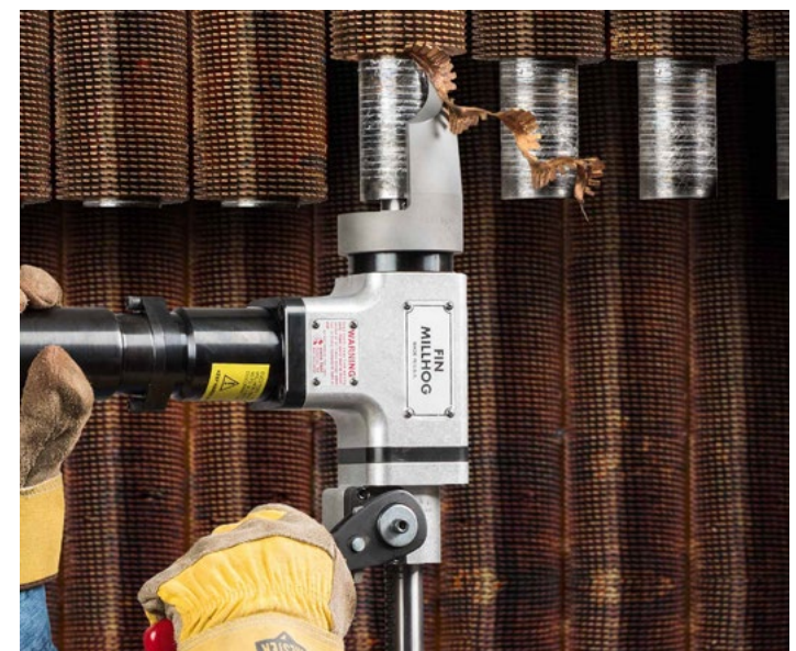
The FIN MILLHOG® rack and pinion feed has a 4.0" of stroke that allows the operator to quickly engage and disengage the cutter for clearing separated fin from the work area.
