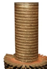
4.0" (101 mm) depth of fin is removed and tube is ready for beveling.
