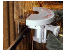
The boiler tube panel saw works on the same track as the straight-thru models.
