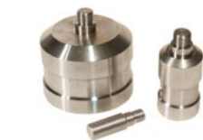
Pilots center the tool and keep it square to the tube. A properly sized pilot is .015" to .030" under the tube I.D. This tolerance ensures smooth operation, long blade life and chatter free bevels.
