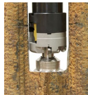
Remove membrane and overlay/cladding from between tubes
