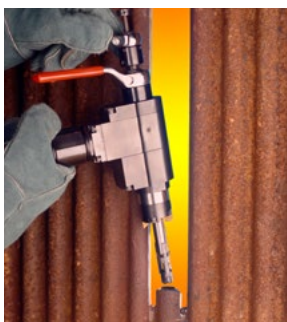
Only 1.5" wide for single boiler tube beveling
