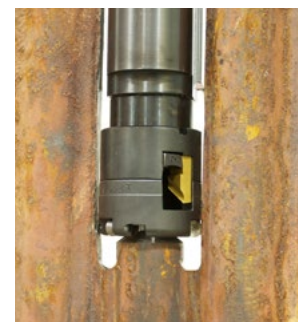
Remove membrane from between tubes
