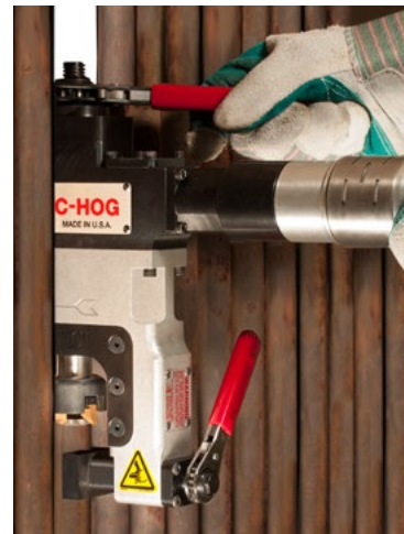
This rugged tool has a narrow profile and can fit between 1.25" O.D. membrane water wall boiler tubes to bevel a single tube for a Dutchmen tube repair.
