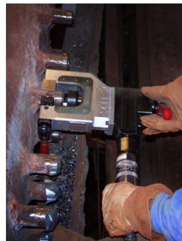
The C-HOG is ideally suited for beveling small bore heavy wall tubes with a high percentage of chrome, stainless steel and other hard alloys.
