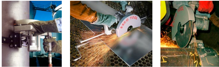
The Standard APS can also achieve perfect cuts on contoured and cylindrical structures, steel plate and pipe from 6.0" to 60.0" with available accessories.
